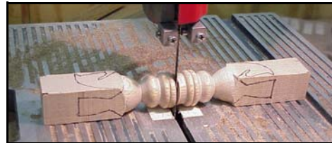
Fig. 13 Cutting the Knights off at the base
