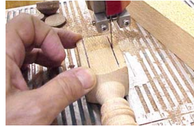
Fig. 11 Cutting a 1" square in preparation to cut the Knight
