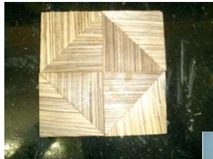
Figure 4. Blank made by gluing corners
